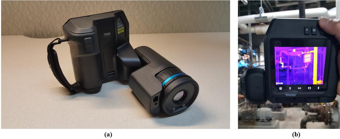
Figure 7 – (a) FLIR T540 professional thermal camera; (b) data collection in scene 1
