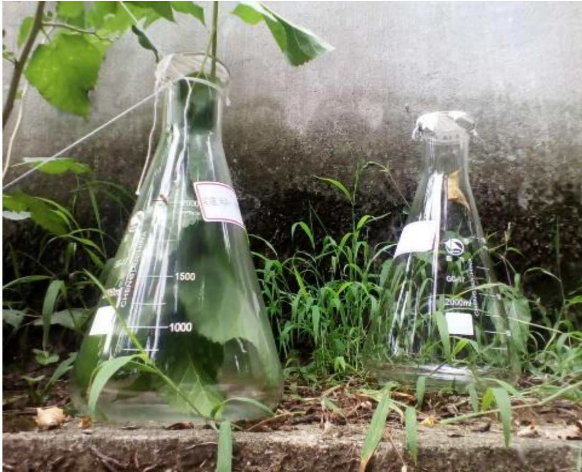
FIGURE 2-1: Static headspace aeration method of Morus alba foliage and a blank control (both in 2L Erlenmeyer flasks) (Nanjing, China, 2017). Photo taken by author.
