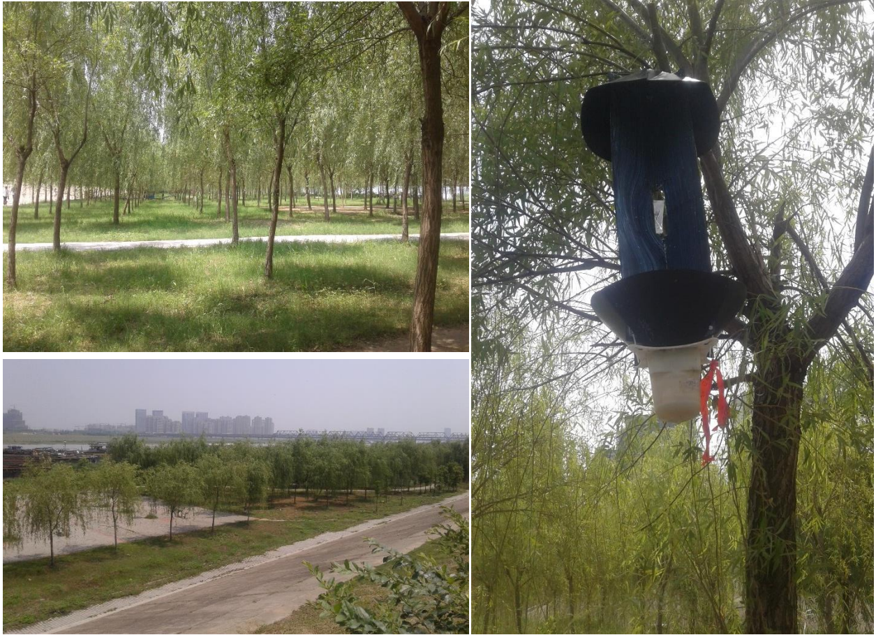
FIGURE 3-1: Bengbu Trapping Location Vistas and hung Black Intercept Panel Trap. (Photos taken by author, Summer 2018).
