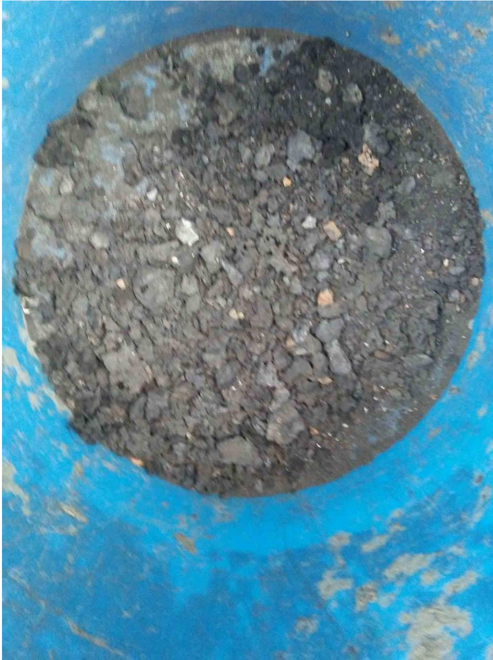
Figure 23. Ash and biochar collected from the ash pit and cyclone
