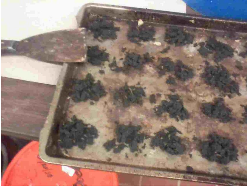
Figure 11. Biosolid fuel after oven drying
