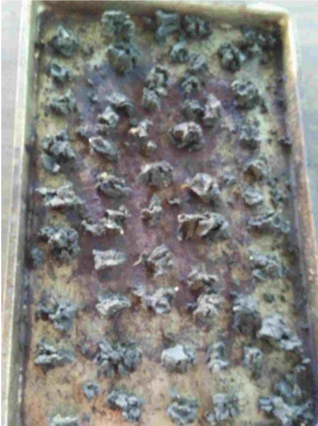
Figure 15. Dried Pressed Biosolids with no Hemp Fiber
