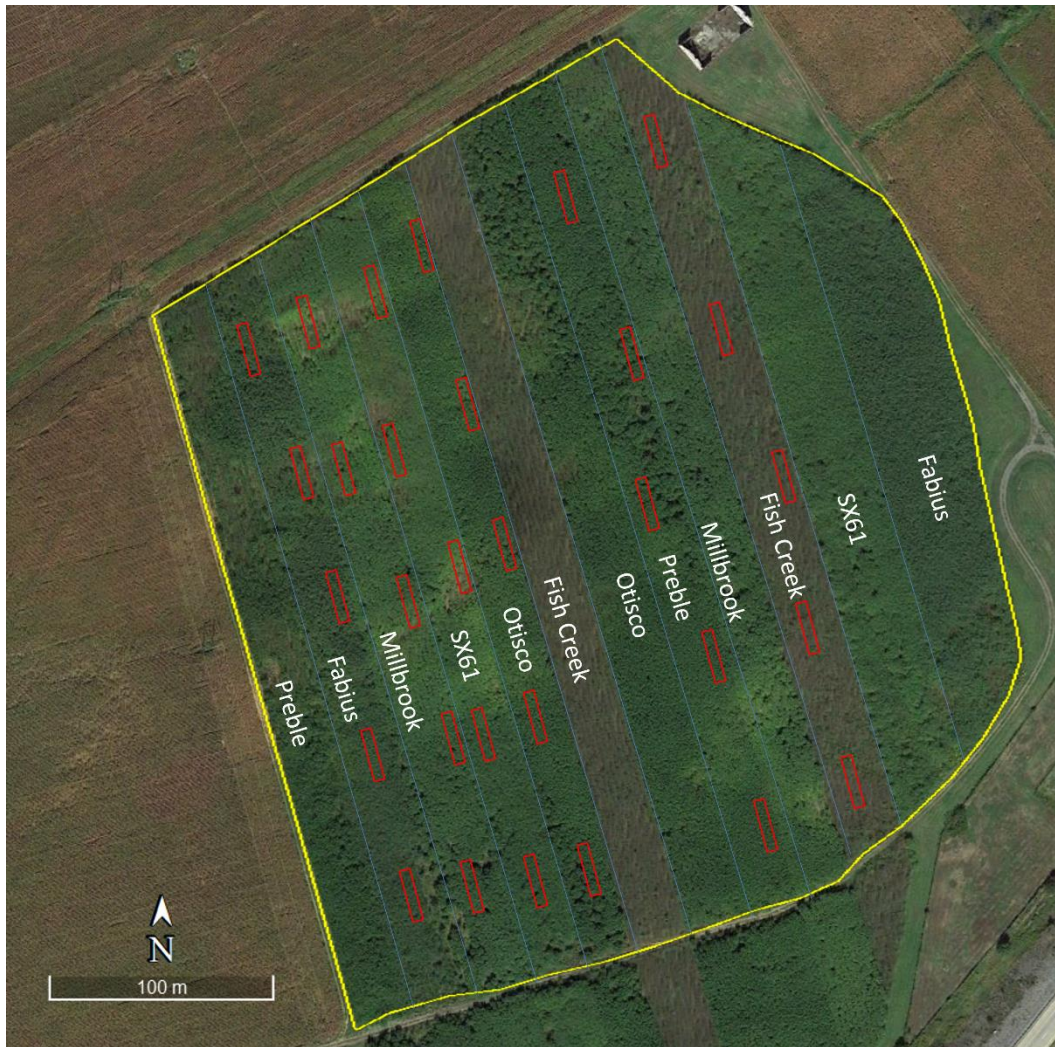
Figure 4.1. Outline of the selected area at the site (yellow line) where hand harvesting and machine harvesting data were collected to assess biomass and nutrient losses. Measurement plots (red lines) were installed in each randomly selected double row and were spaced along the length of the rows for each cultivar (delineated by white lines).
