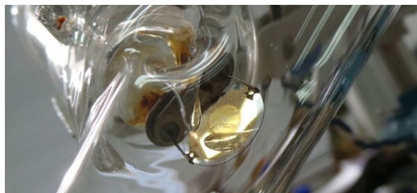
Fig. 4. Photograph illustrating the presence of a residual organic sample on the plate surface at the end of stage F
