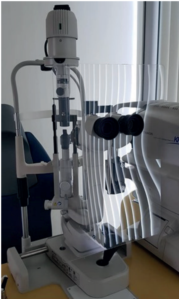
Fig. 1. Protective shield for biomicroscope, providing full separation between the patient and the doctor.
