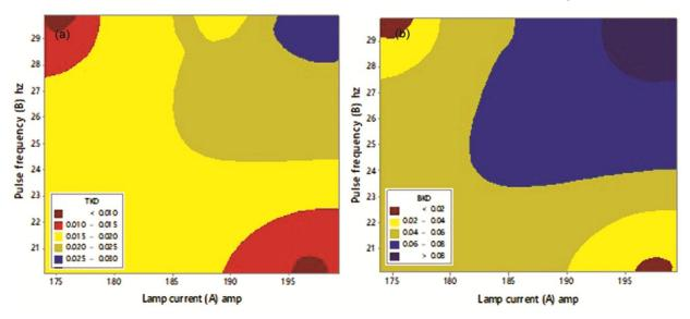
Fig. 4 — Stable cutting zone for (a)TKD and (b) BKD, when C, D and E are fixed
