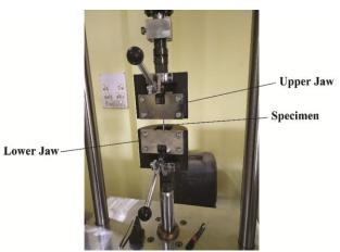
Fig. 2 — Universal testing machine
