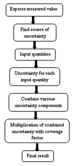
Fig. 1 — Steps to calculate uncertainty of measurement using LPU/ GUM  $^{9\text{-}12}$
