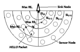
Fig. 3 — Reserve Route Request processing through query hello packet
