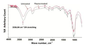
Fig. 3 — ATR-FTIR spectra of untreated crosslinked and plasma-treated crosslinked linen fabrics
