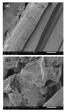
Fig. 2 — SEM images of (a) untreated crosslinked and (b) plasma-treated crosslinked linen fabrics
