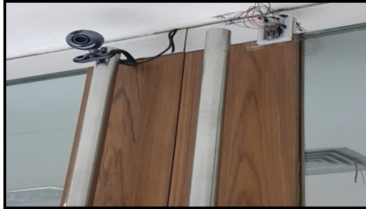
Figure 6. ARDUINO-BASED OFFICE SECURITY SYSTEM PROTOTYPE USING FACE RECOGNITION FEATURES
