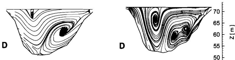
Figure 2. Streamlines showing secondary circulation in the cross-section D – grid sensitivity analysis. Results obtained for the coarsest grid (left) and the finest grid (right)
