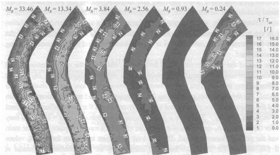
Figure 4. Contour lines showing change in the non-dimensional bed shear stress distribution with respect to the change in the  $M_R$  value at the confluence ( $d = 0.28$  mm)
