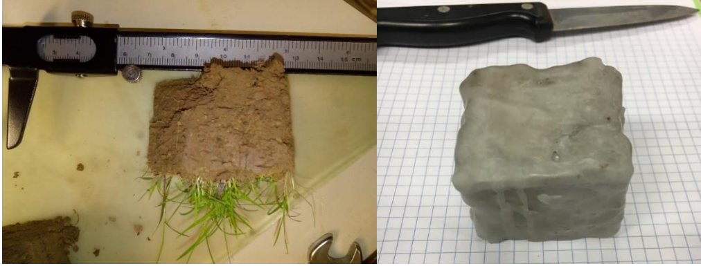
Figure 36 Paraffin tests on vegetated soil: before and after soil covering
