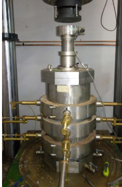
Figure 34 triaxial cell and horizontal LVDT supports used in the investigation.
