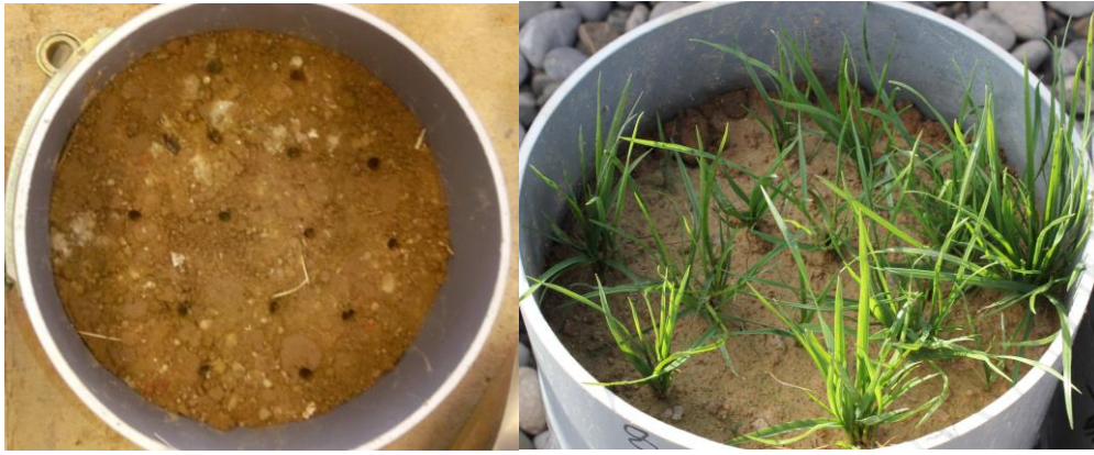
Figure 30 Plants seeding in 40 mm spaced holes and after growth in moulds
