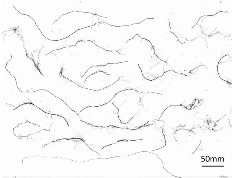
Figure 31 a) roots retrieved from soil sample, b) pycnometer test to calculate roots volume, c) WinRhizo scan to evaluate roots geometrical properties (diameter, length).
