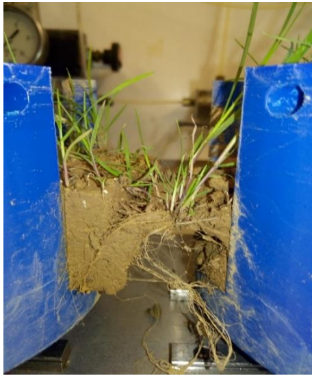
Figure 44 Unbroken roots after test, within the fissure generated by the tensile test
