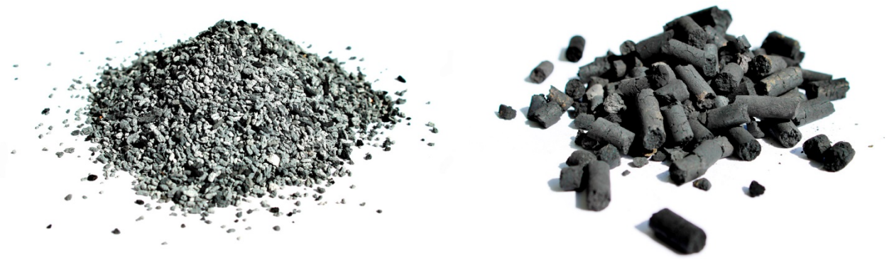
Figure 10. Two different ashes produced from the same sewage sludge substrate by thermal gasification in a low-temperature circulating fluidized-bed gasifier (left) and a two-stage downdraft gasifier (right).
