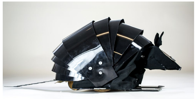
Figure 10. A customized version of the Animism Robot with embedded Anthropomorphic behavior.
