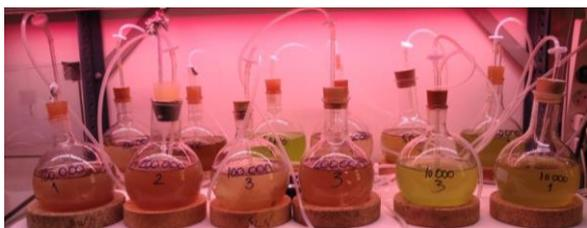
**Figure 6.** 1 L balloon flasks used for cultivation for some of the small-scale experiments with *Rhodomonas salina*. The flasks are equipped with tubes for filtered aeration (0.2  $\mu\text{m}$ ).
