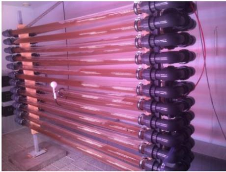
**Figure 8.** The tubular PBR (250 L) during a meso-scale experiment with *Rhodomonas salina*. (Photo: C. Thoisen)
