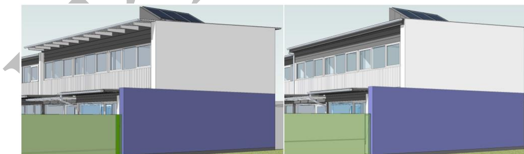
Figure 4. Design with roof overhang (left) and without (right). Model made by Martin Rubow, Architect MAA, and Carl Galster, Architect MAA.
