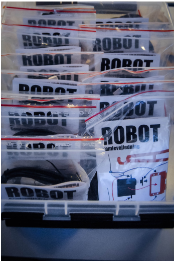
Figure 9: The robot kits are designed as products to be inviting and provide both initial success and later hackability. They are mass produced with basic laser cutting materials.
