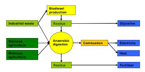
The system illustrated above combines two biofuel production lines. One that converts slaughterhouse waste (fat) into biodiesel and a second one which use the slaughterhouse waste directly in the biogas reactor. The two systems can also be combined in a system in which the residue (glycerine) from the biodiesel is utilised in the biogas plant. The use of the residue from the biodiesel production will be determined by the market price for glycerine as glycerine is also used in competing products.
