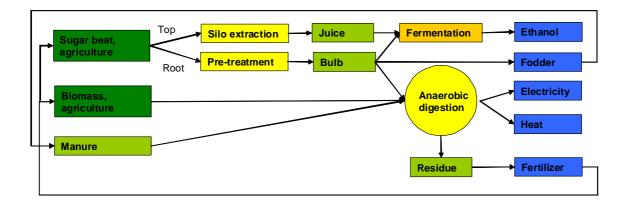
The concept illustrated above includes a decentralised silo storage system for the sugar beet top. The root is pre-treated at two stations. The root is first cut into small pieces and afterwards pressed. The juice which is rich in sugar can then be fermentated into ethanol in a low cost 1. generation system that renders the use of expensive enzymatic treatment obsolete. The residue from the bulb can subsequently be used as animal feed or as input for the biogas plant.
