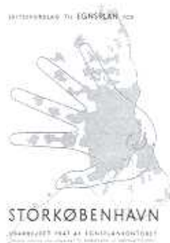
Figure 1. The original sketch of the 1947 Fingerplan of Copenhagen. The palm is resting on the city centre of the 1940's. The fingers point in five directions, the shaded areas represent both existing and future cities. To the north the existing urban fabric did not fit completely to the little finger, as these areas were already under development.
