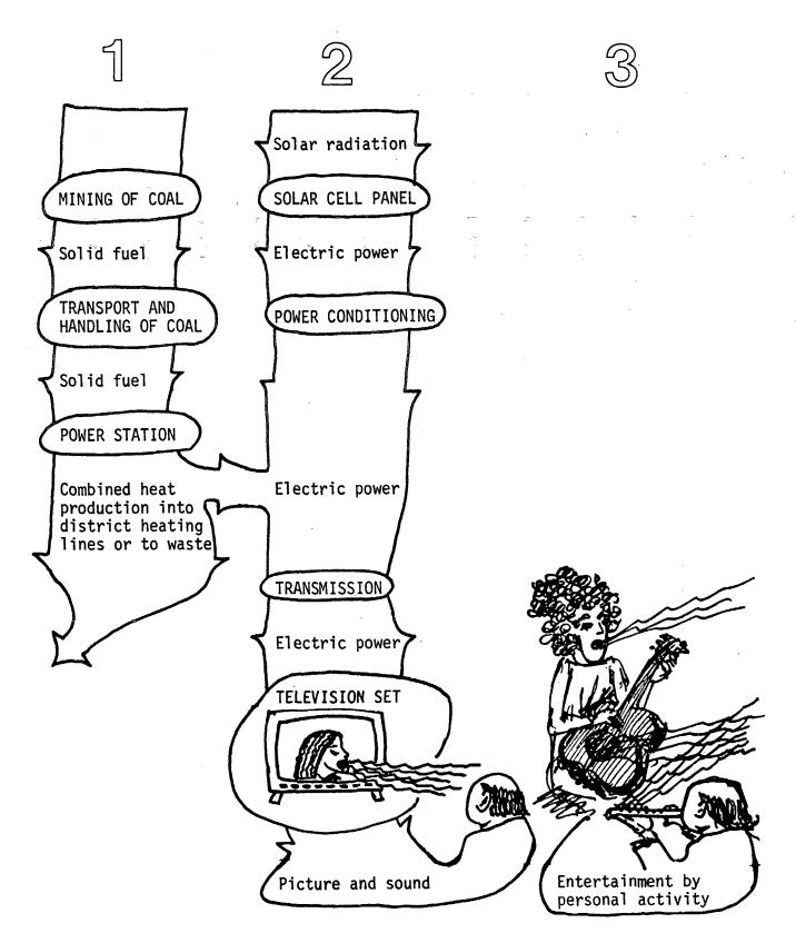
Equipment characterized by a definite technical efficiency is circled.
