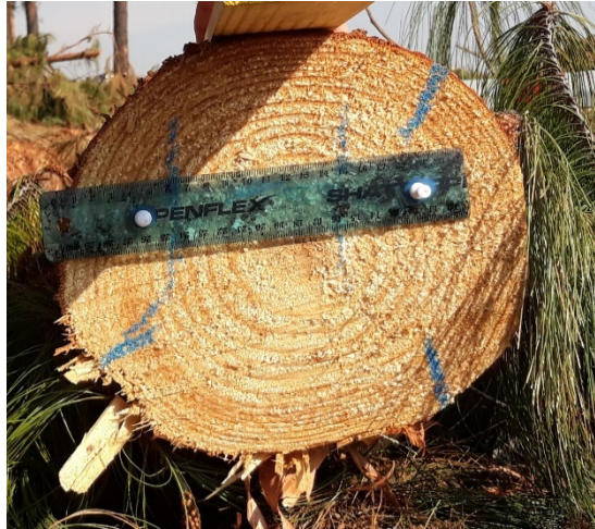
Figure 6: Log end photograph with the log ID code and ruler used to scale photograph for photogrammetric analysis.
