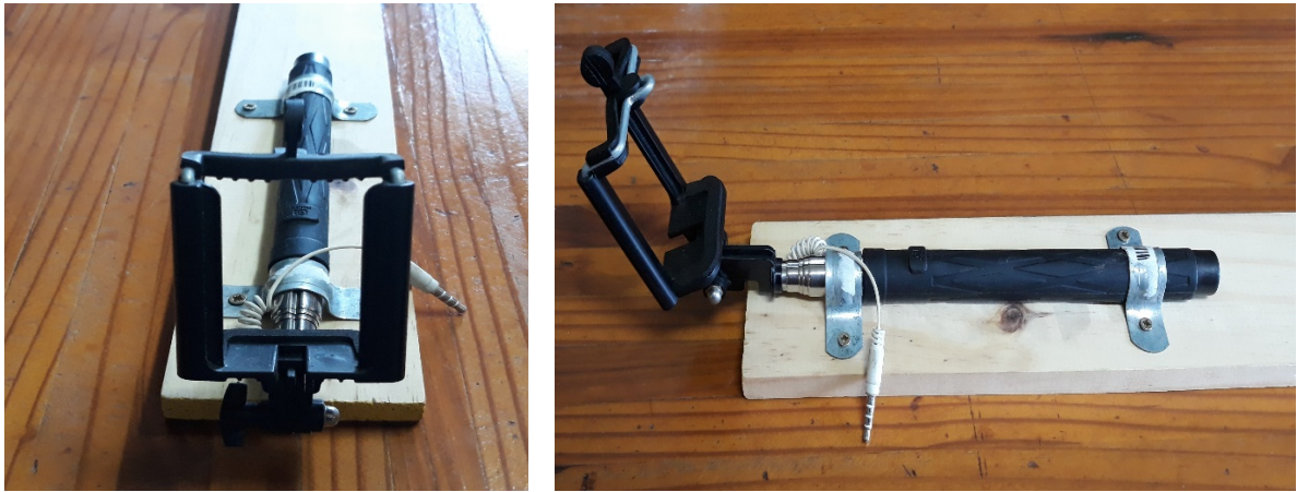
Figure 2: Photography rig used to take photos of the log small ends and stumps.
