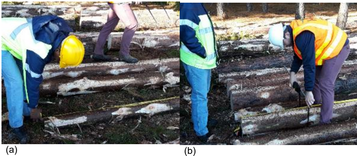
Figure 5: The manual length (a) and diameter (b) measurements done for the calibration process.
