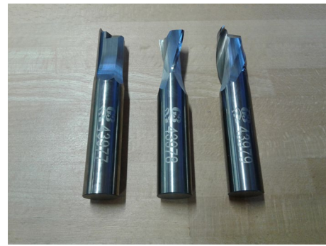
Fig. 2 Mills used during the cutting experiments, from left to right: straight blade, 15°-helical cutter, and 30°-helical cutter
