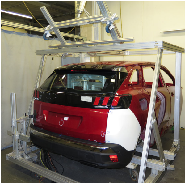
Fig. 17 Durability test on tailgate 3008
