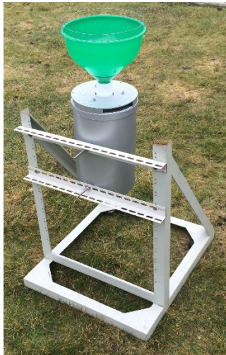
Figure 6 The Palmex rain sampler RS1, equipped with the 23 cm funnel.
