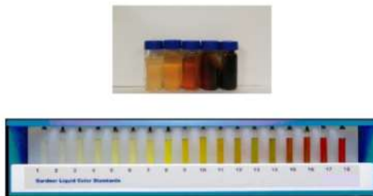
Figure 4. Colour of the product samples produced at different reaction temperature (from left 140°C, 160°C, 180°C, 200°C and 220°C) and Gardner scale model
