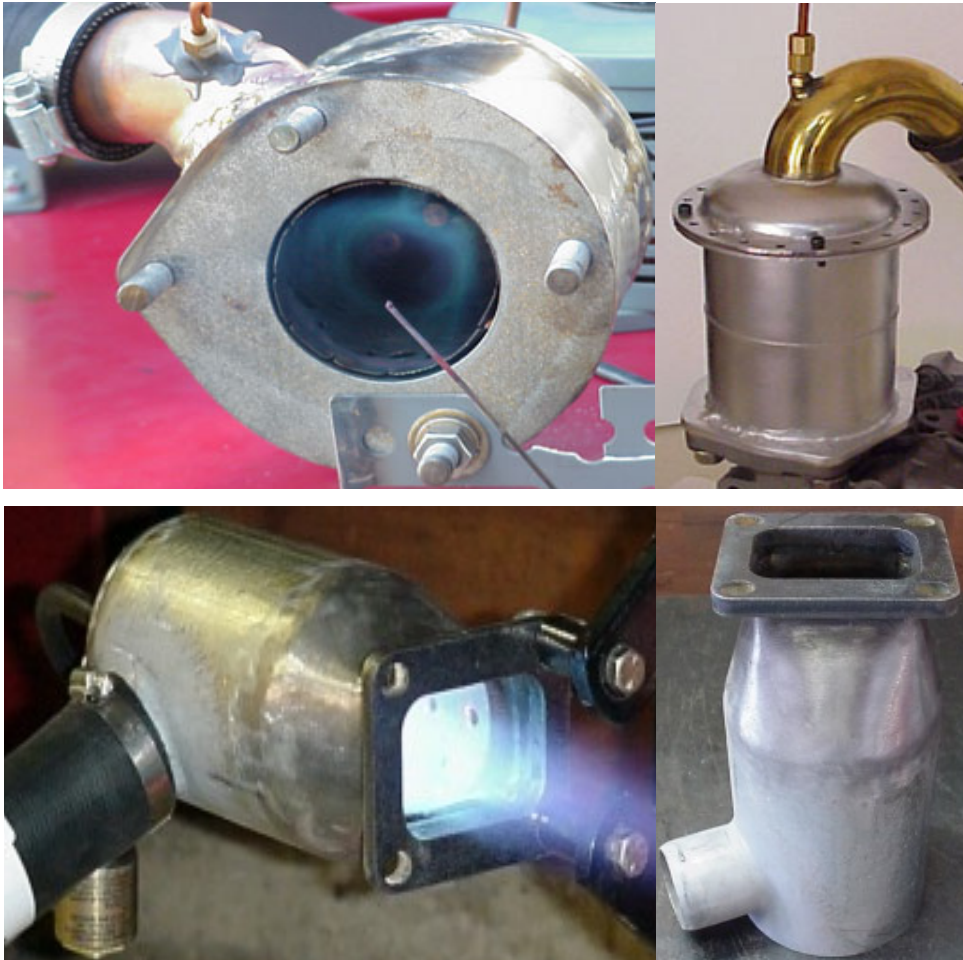
Figure 2.3.3.10 Side-entry combustors by: Mike SJet (top); RCDon (bottom) [84], [85]
