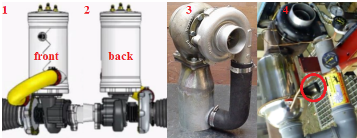
Figure 5.1.1 CAD and actual depictions of side-entry (1, 2, 3) and axial (4) combustor on a turbocharger
