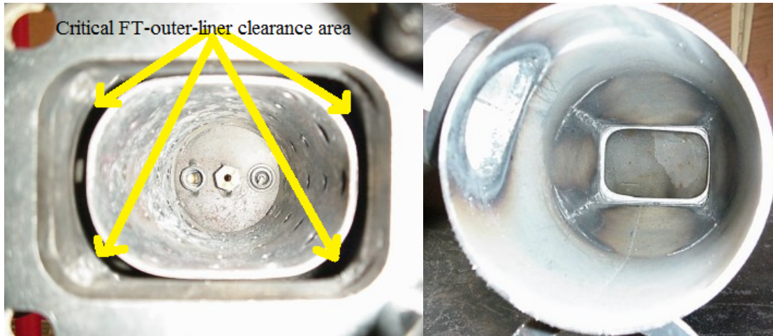
Figure 5.1.6 Top-end (l) and open-base (r) views showing internal orientation of the SEC
