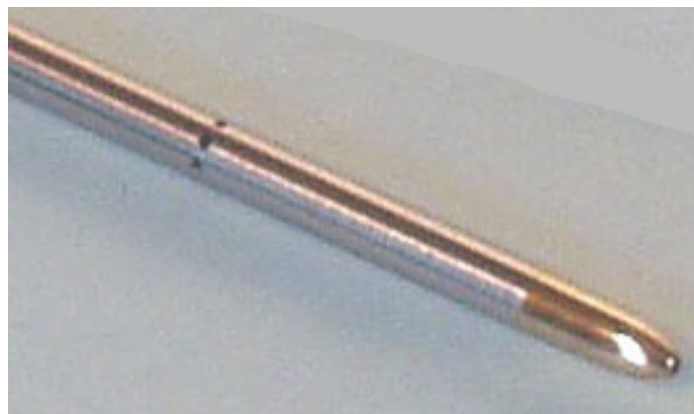
Figure 5.3.1 Pitot-static or Prandtl tube
