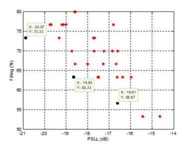
**Figure 5.** Convergence curve of PSLL versus array filling of 30 trials with CTF crossover rule. The red marker is PSLL value versus array filling for 27 individuals. A black marker is the best of three individuals based on the lowest PSLL and array filling.
