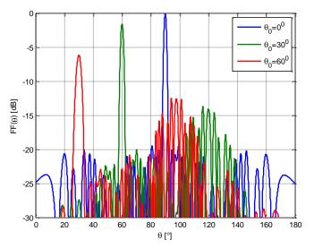
Figure 10. Scanning the far-field pattern from Figure 9 (a) at the angle of  $0^{\circ}$ ,  $30^{\circ}$ , dan  $60^{\circ}$ .
