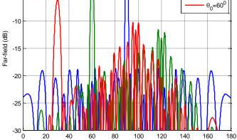
Figure 7. Scanning the far-field pattern from Figure 6(a) at 0°, 30°, dan 60°.
