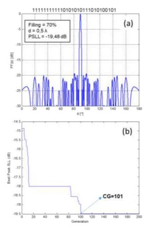
**Figure 9.** (a) Far-field pattern for CUP antenna based on PTT rule with 70% turned ON elements, and PSLL is -19.48 dB in trial #2. (b) Convergence curve of generation versus best PSLL for the same trial.
