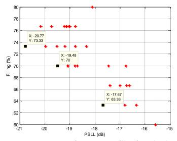
**Figure 8.** Convergence curve of PSLL versus array filling of 30 trials with PTT crossover rule. The red marker is PSLL value versus array filling for 27 individuals. A black marker is the best of three individuals based on the lowest PSLL and array filling.
