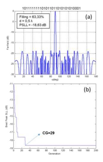
**Figure 6.** (a) Far-field pattern for CUP antenna based on CTF rule with 63.33% turned ON elements and PSLL of -18.63 dB in trial #18. (b) Convergence curve of generation versus best PSLL for the same trial.
