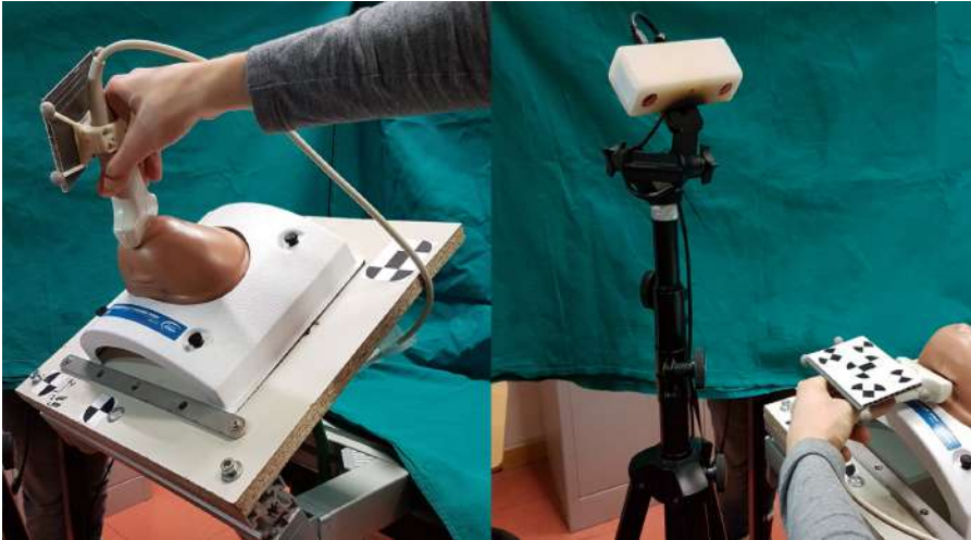
Fig. 6 The multi-modality setup uses an optical tracker and markers that define a reference system attached to the breast phantom. The US probe is tracked as well.
