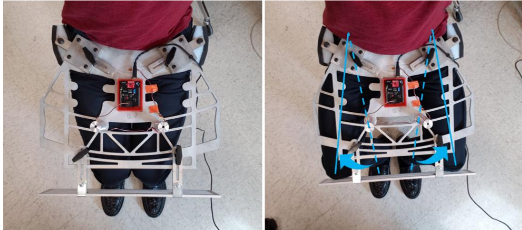
FIGURE 14 – A top view example of an abduction performed from the starting position (left) to the peak abduction into the pads (right) where the blue represents the approximate motion of the femur about the acetabulum.
