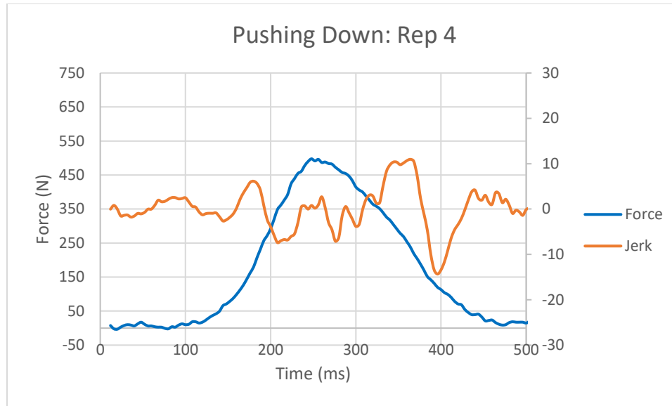
FIGURE 31 – An example force and jerk graph over time of a standard rep while pushing down onto the plate.
