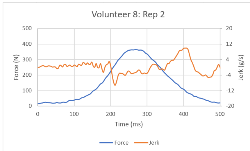
FIGURE 35 – Example dynamic volunteer data showing a typical force curve with the minimum jerk peak as force increases.
