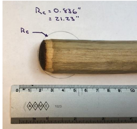
Figure 11: The spindle-divot interface is very nearly spherical in shape.
