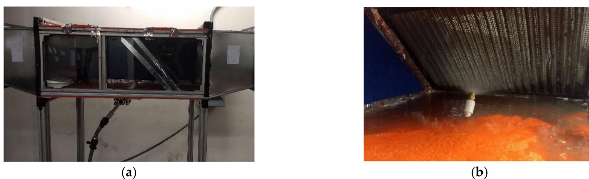
Figure 1. (a) Set-up for installation of dust filters for performance testing; (b) fibrous dust filter with water spray operational.
