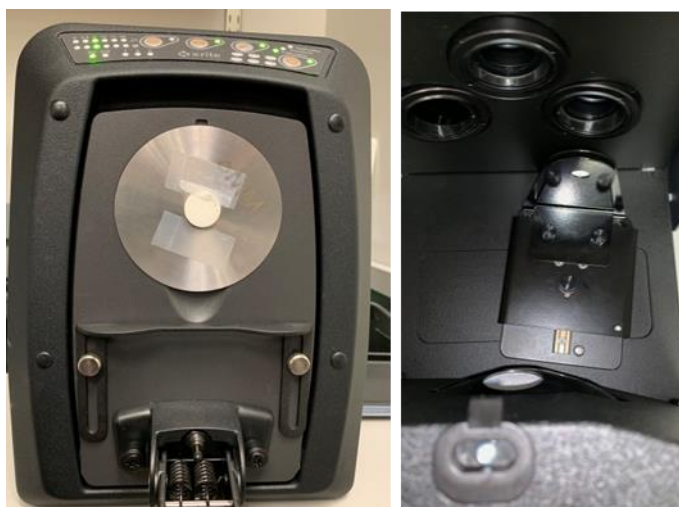
Figure 3.13 A PICN specimen in place to measure CR and TP (left). For the LT measurement, the specimen was fixed with a holder and aligned against spherical lens.
