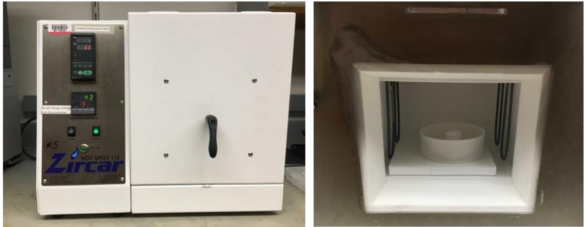
Figure 3.3 Zircar Hot Spot furnace was used for sintering of alumina matrices.
