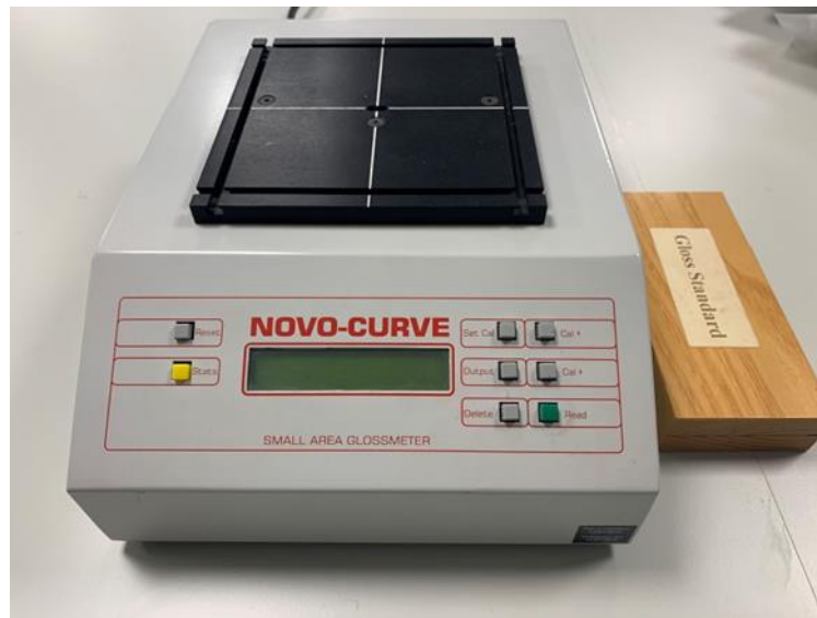
Figure 3.25 A calibrated Novo-Curve was used to measure the gloss of the test materials.
