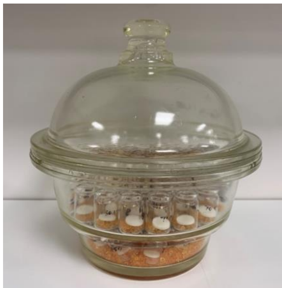
Figure 3.26 Desiccator showing the samples stored in separate glass vials with anhydrous self-indicating silica gel at the bottom prior to immersion in water and artificial saliva.
