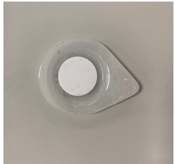
Figure 3.22 A pre-heated silica crucible containing a PICN specimens before (left) and after burn out (right).
