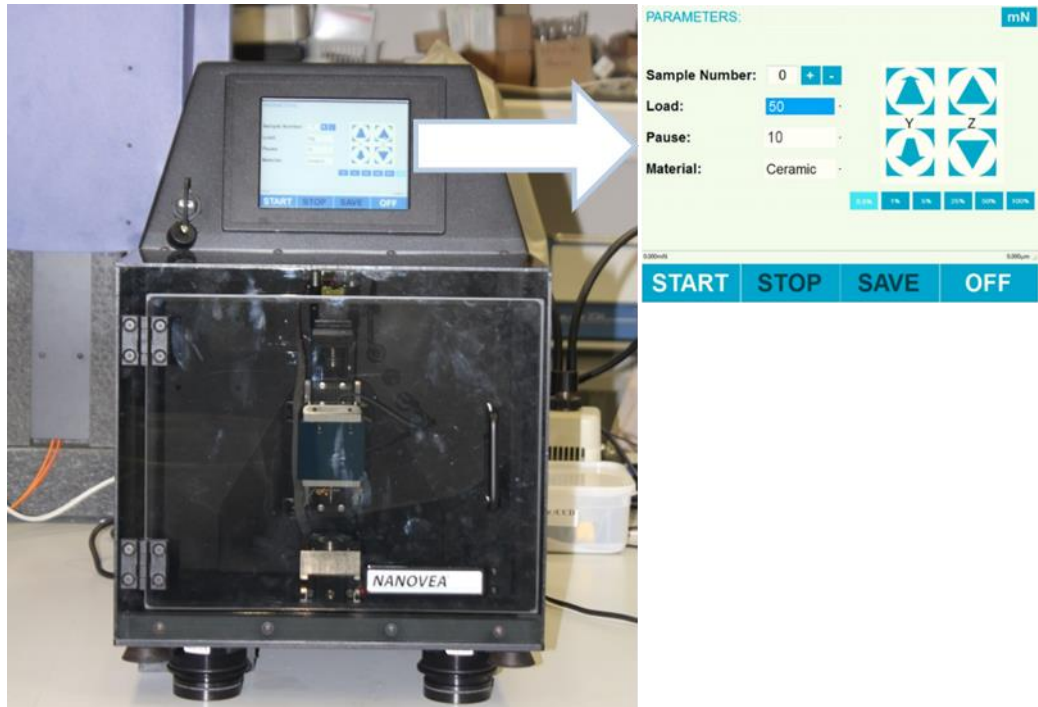
Figure 3.18 Nanovae indentation device with the selected test parameters used to examine the CAD/CAM ceramic specimens.
