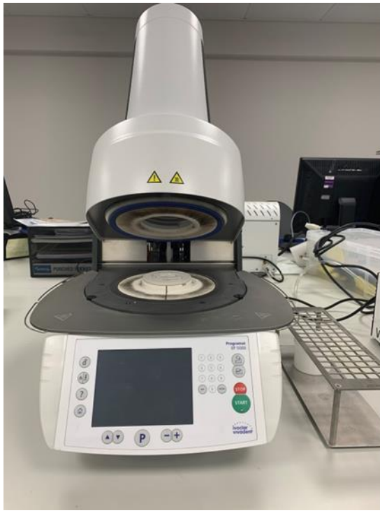
Figure 3.21 Programat electric furnace was used to burn out the specimens (left) which were weighted before and after the burn out using calibrated analytical balance (right).
