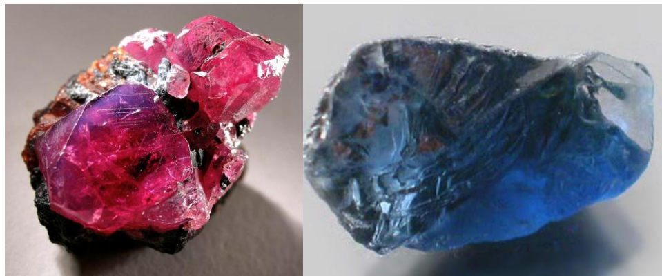
Figure 1.6 Two forms of alumina precursors (Corundum), ruby (left) and sapphire blue (right) depending on the doping elements present.
