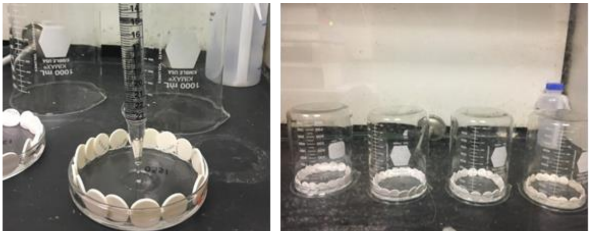
Figure 3.6 Specimens were arranged into a plastic dish and were half-height soaked into silane for 3 hours in laboratory fume hood.
