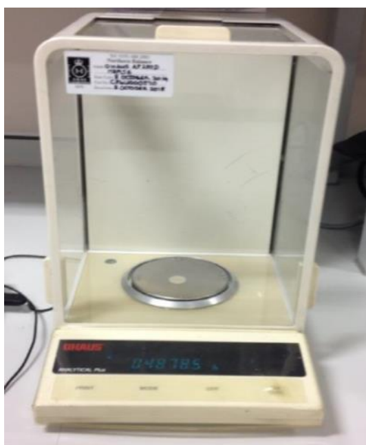
Figure 3.27 Electronic analytical balance used for weighing the test samples (Ohaus Analytical Plus, Ohaus Corporation, USA).
