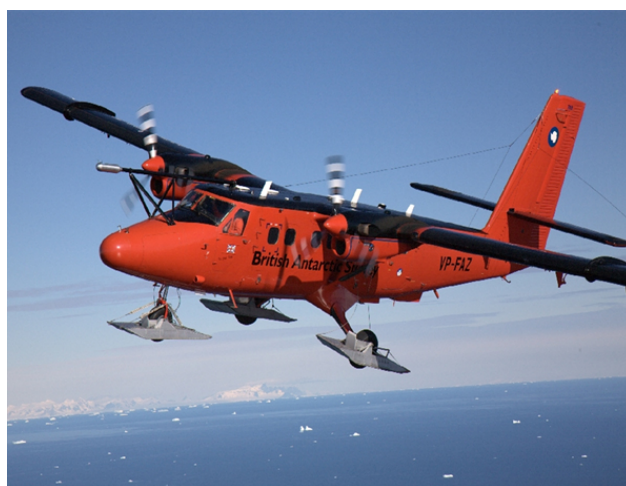
Figure A2. Photo of the BAS Twin Otter showing the turbulence boom protruding from the front of the aircraft superstructure.
