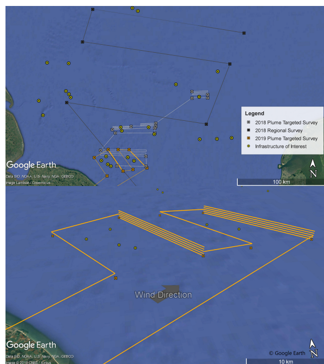
Figure 3. The top panel shows flight patterns of the regional and plume capture styles of flight deployed between 2018 and 2019, alongside infrastructure of interest (such as drilling rigs, gas distribution platforms or production platforms). The bottom panel shows a 2019 plume sampling survey of idealised stacked transects in the 2D plane downwind of infrastructure of interest. © Google Earth 2019 for background imaging.
