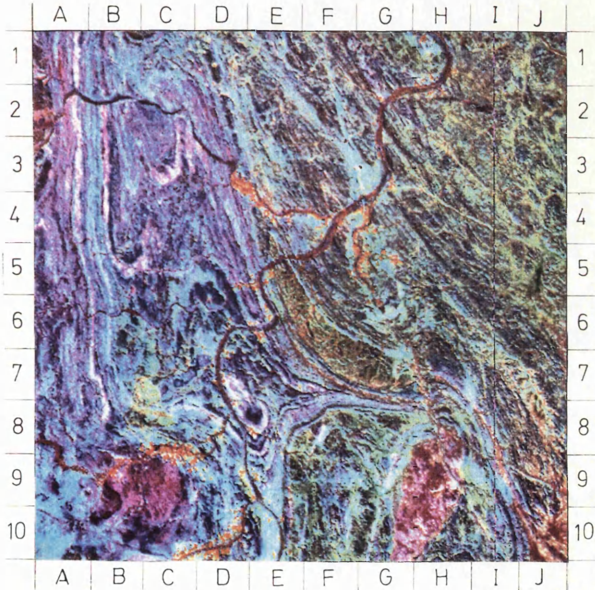
Fig. 3.4 A contrast-stretched CRC of TM band 5/7 in red, band 5/1 in green, and band (5/4x3/4) in blue for the test-site No.1.
