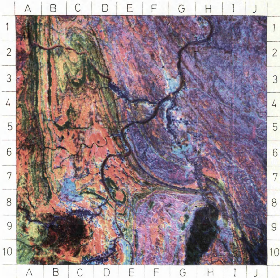
Fig. 3.8 Linearly contrast stretched CRC of TM band 7/5 in red, band 5/4 in green, and band 4/2 in blue for the test-site No.1.
