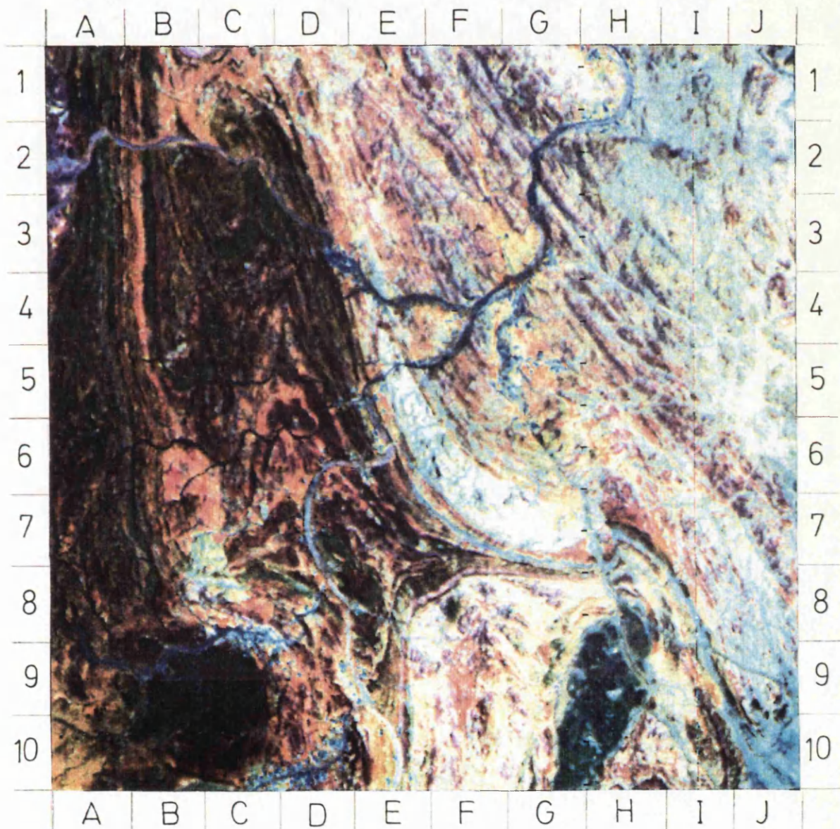
Fig. 3.9 TM band 7,5,4 red,green,blue scaled decorrelation stretched FCC image for the test-site No.1.
