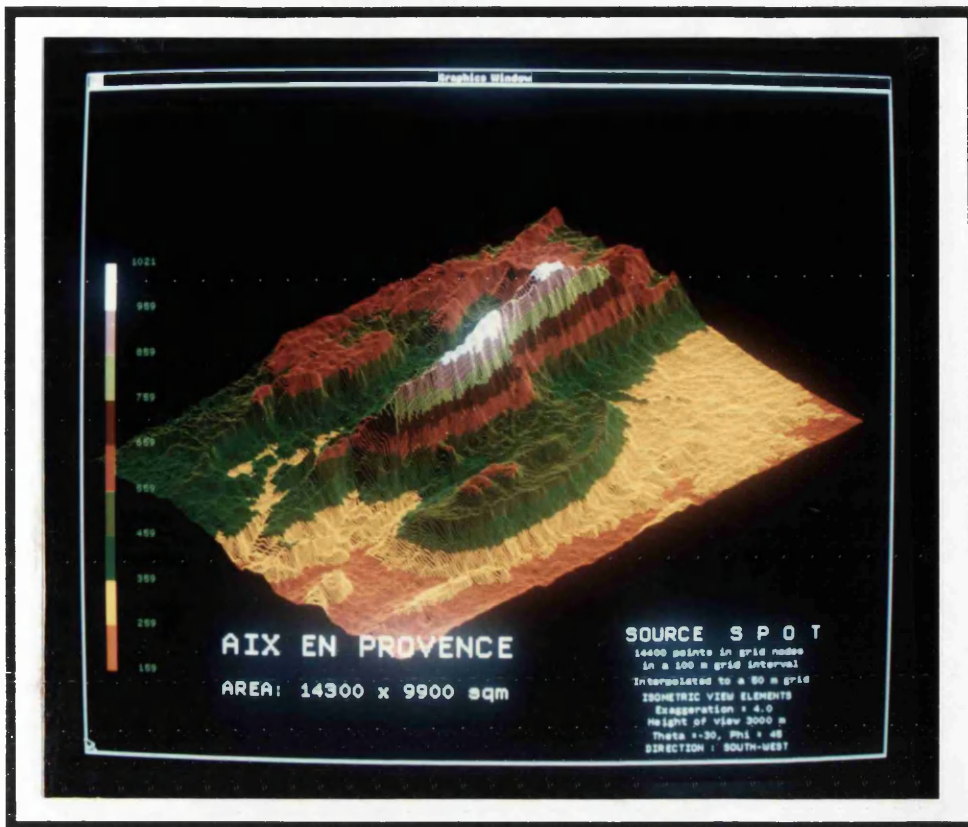
Plate 9.3. Isometric view of the SPOT DEM from South-West direction
