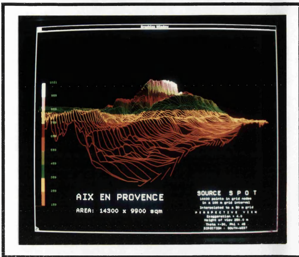
Plate 9.1. Perspective view of the SPOT DEM from South-West direction (height of view 250 m above sea level)
