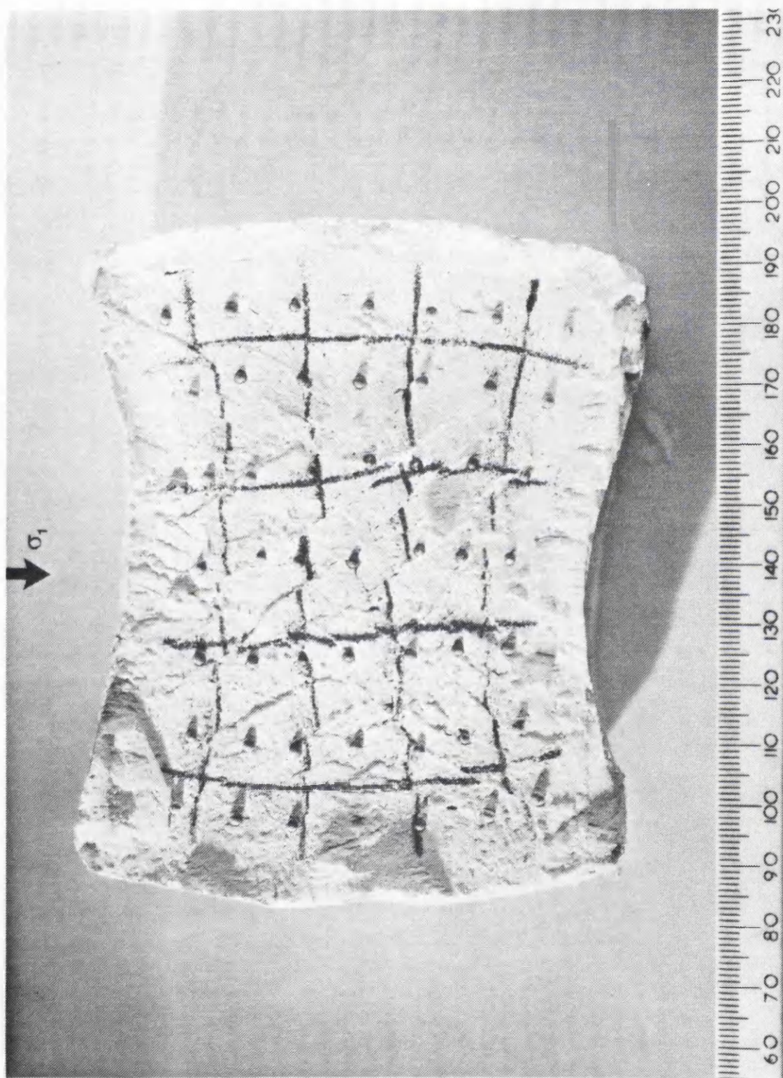
Fig. 7.49 Coulomb slips in nearly saturated kaolinite sample sheared monotonically in plane strain in the DSC without the shear sheets around the sample with \psi = 90^\circ
