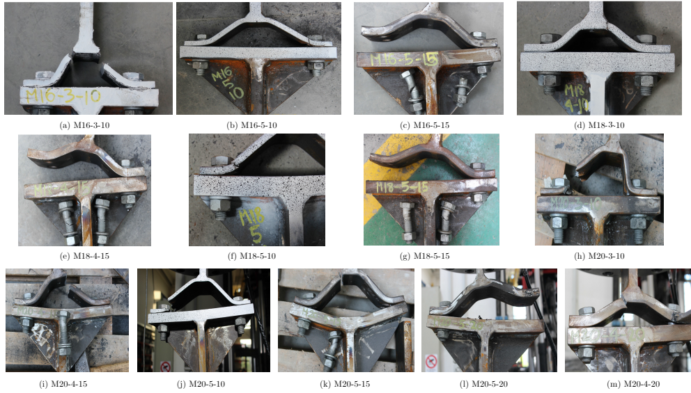
Fig. 5: Post-test (failed) specimens - see Table 2 for the classification of their failure mode.
