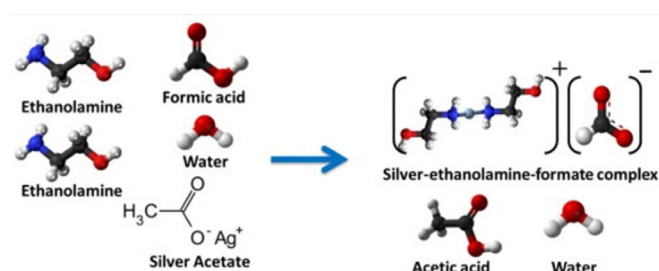
Figure 2. Chemical reaction involved in the formulation of Vaseem et al.'s ink. Adapted with permission from ref. [24], Copyright 2016, Elsevier.
