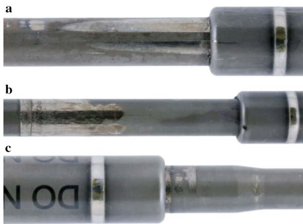
Fig. 6 Examples of different wear patterns in explanted MAGEC rods
