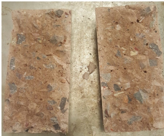
Fig. 14 Failed cylindrical specimen
