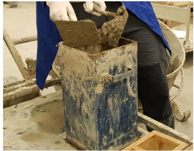
Fig. 7 Filling mould with fresh concrete
