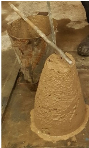
Fig. 6 Laboratory slump test
