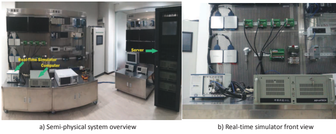
Fig. 6: Semi-physical testing environment
