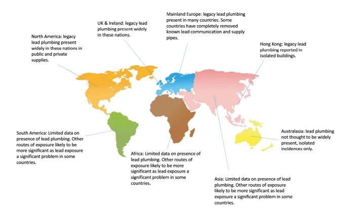
Figure 1. Presence of lead plumbing in water supply systems across the world.
