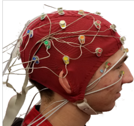
Figure 3. 8: A study participant wearing 32 channels EEG devices with electrodes covering the whole scalp [245].
