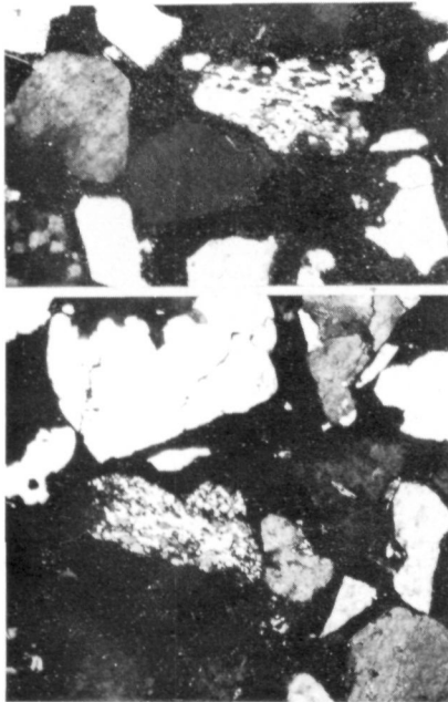
Fig. 50. Moderately sorted, sub-angular quartz grains embedded in cryptocrystalline dark matrix with interstitial flow structures (quartz arenite, Hienheim 317). 40 \times .
