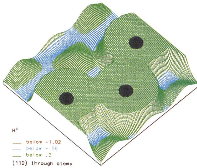
FIG. 6. Perspective plot of the energy surface for H^+ in a (110) plane through the Si atoms. To generate the values for this plot (unlike all others) the Si atoms were kept fixed in their rigid lattice positions. Comparing with Fig. 3, we see that the low-energy regions have disappeared.
