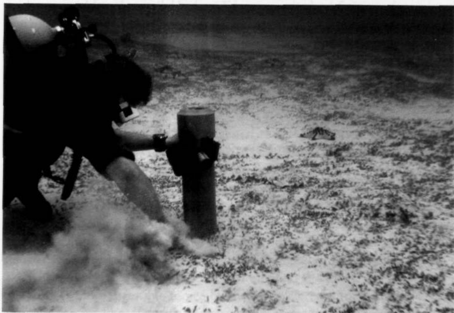
PVC corer used during scuba diving to take seagrass samples at grazing swards of dugongs
