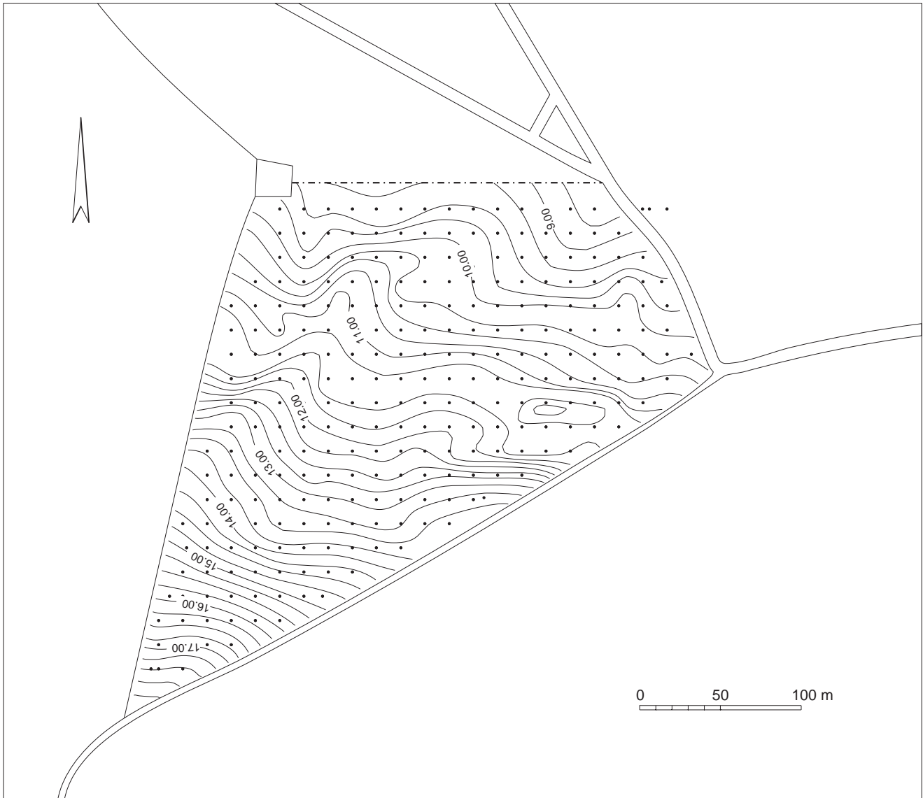
Fig. 2.3. The location of the auger tests in the survey area.
