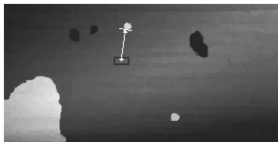
Fig. 9. 2495 \times 1248 \text{ \AA}^2 STM image of the Cu(001) surface at 343.3 K. The surface area that was selected to perform the diffusion measurements at this temperature is indicated by the rectangle. The trajectory to the nearest step has been drawn in the figure. The length of this trajectory is shown in Table 2 ( V_t = -1.16 \text{ V} , I_t = 0.1 \text{ nA} ).
