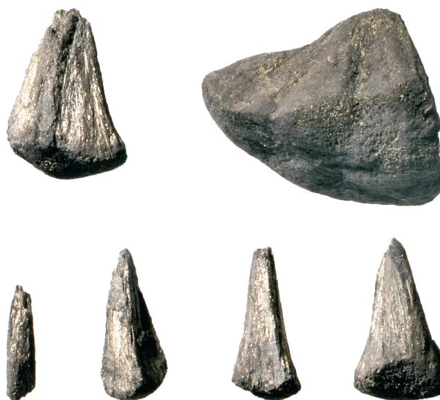
Figure 8.11 Fragments of pyrite nodule, mostly of radial pyrite. Some of the pyrite has crumbled (magnification 2x).
